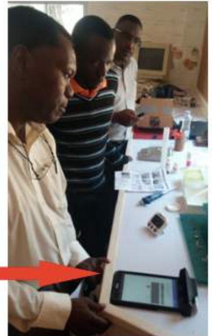
Figure 2. (Left) Asus MemoPad 8 HD case and illumination hood holding the aflatoxin test strip adapted from the provisional patent MODULAR ILLUMINATION AND SENSOR CHAMBER. (Right) Zambia Ministry of Agriculture testing Aflatoxin using the 3D printed case and holder.
