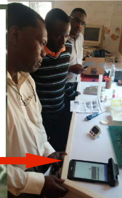
Figure 2. (Left) Asus MemoPad 8 HD case and illumination hood holding the aflatoxin test strip adapted from the provisional patent MODULAR ILLUMINATION AND SENSOR CHAMBER. (Right) Zambia Ministry of Agriculture testing Aflatoxin using the 3D printed case and holder.
